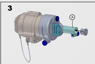
Place the appropriate laser adapter into the laser aimer holder (A).
