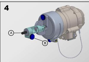
Insert the laser into the laser adapter (A) and tighten the holding screw (B).
