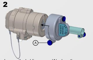
Loosen the holding screw (A), place the cone viewer on the detector and tighten the holding screw (A).
