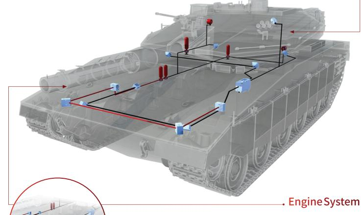
The engine compartment fire protection system is designed primarily to detect accidental slow growth type fires such a fuel leaks and overheating conditions. An engine fire protection system that responds in several seconds will prevent catastrophic destruction of the vehicle.
